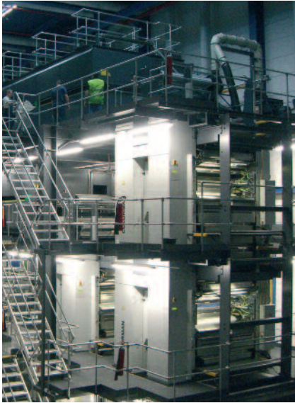
Printing presses with larger formats and direct drives require less energy and produce less waste. Photo manroland.
