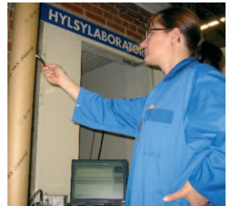
E-modulus quality control measurement - a high E-modulus and low density reduce the risk of a core break. Photo Sonoco-Alcore.
