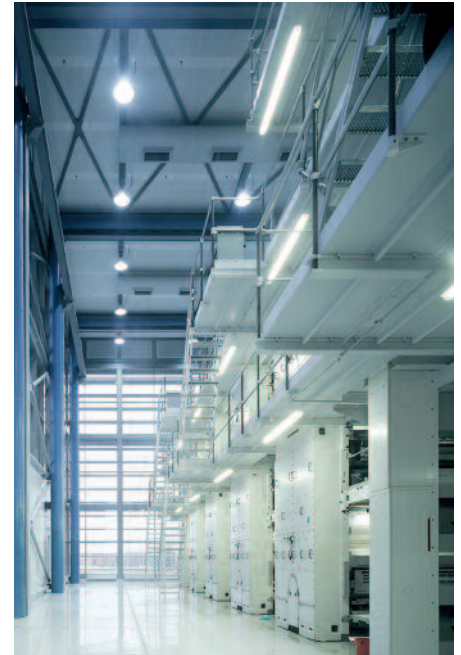
The press hall ensures maximum natural daylight plus efficient artificial lighting for night working. Excessive heat build-up from the press, auxiliary equipment and lighting was avoided by ensuring efficient thermal flows within the building.
