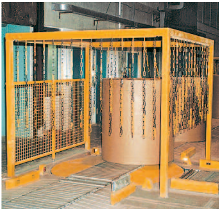
Conveyors will need to be able to handle increased roll weight and width, whilst turns require more space. Photo MAN Roland.
