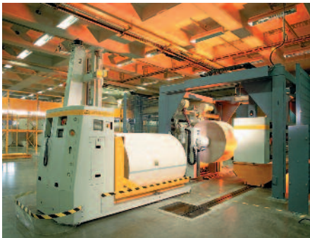
Intermediate transport systems will need a larger capacity to handle increased weight but fewer units may be needed to handle 31% fewer rolls. Photo MAN Roland.
