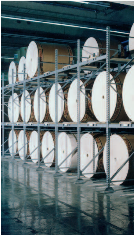
There should be little cost impact on storage for 1500 mm Ø rolls for the same total tonnage as 1250 mm . Photo MAN Roland.
